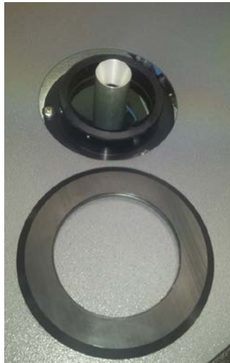
Figure 2-9. Collar for Lower Flange
