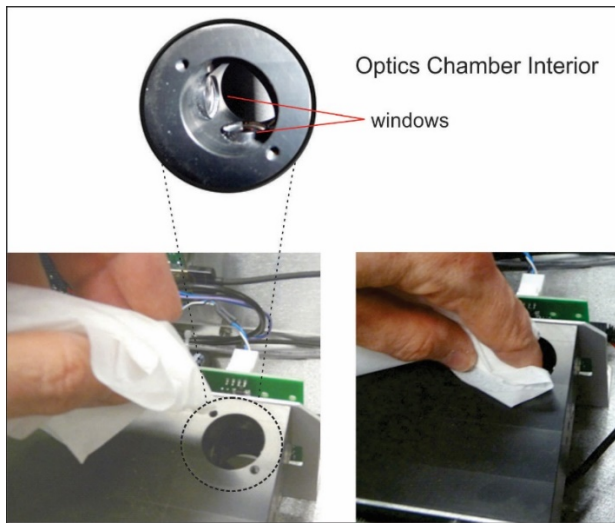
Figure 5-6. Maintenance: Optics Chamber Windows
