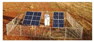
Figure 2. Photo of TAPI T640 (with 640x option) instrument with US EPA approval for  $PM_{10}$ ,  $PM_{2.5}$ , and  $PM_C$  together in a single instrument powered by solar panels. Courtesy: Thomson Environmental Systems Pty Ltd.
