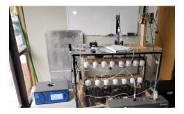
Figure 1. Low-cost particulate sensors being tested alongside a US EPA-approved continuous, real-time ambient particulate monitor. Courtesy: Air Resource Specialists and Colorado State University
