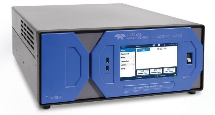
Using IR Gas Filter Correlation technology, the Model T300 CO analyzer produces excellent zero and span stability, high signal-to-noise ratio, and provides advanced electronics to allow accurate, dependable, continuous measurements for ambient air quality, stack gas monitoring and other applications.
