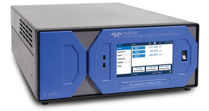
The Model T200U analyzer achieves low level NO / NO<sub>2</sub> / NO<sub>x</sub> measurements using the proven Chemiluminescence principle and advanced electronics. The T200U combines high sensitivity with a wide dynamic measurement range making it ideal for ambient air quality, and other low-level applications.
