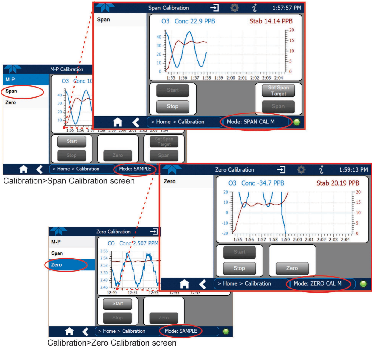
Figure 4-2. Zero and Span Calibration Screens
