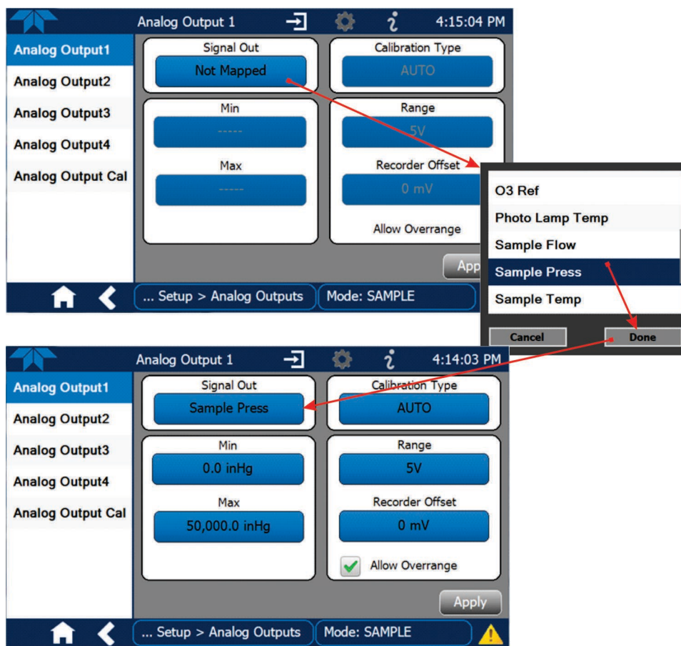
Figure 2-38. Analog Output Configuration Example
