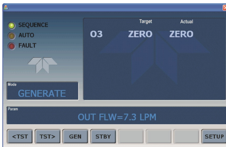
Figure 3-2: Display Screen and Touch Control
