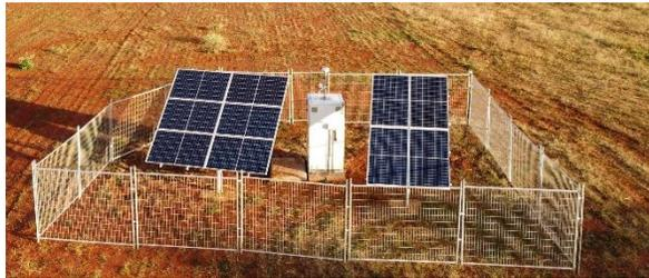
Figure 2. Photo of TAPI T640 (with 640x option) instrument with US EPA approval for  $PM_{10}$ ,  $PM_{2.5}$ , and  $PM_C$  together in a single instrument powered by solar panels. Courtesy: Thomson Environmental Systems Pty Ltd.
