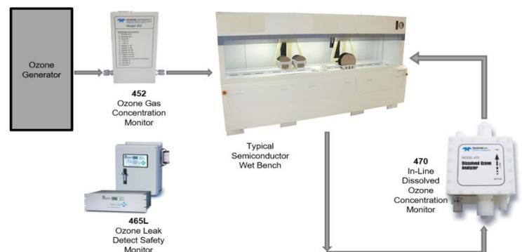
Figure 2: Wet bench system with TAPI ozone instrumentation
