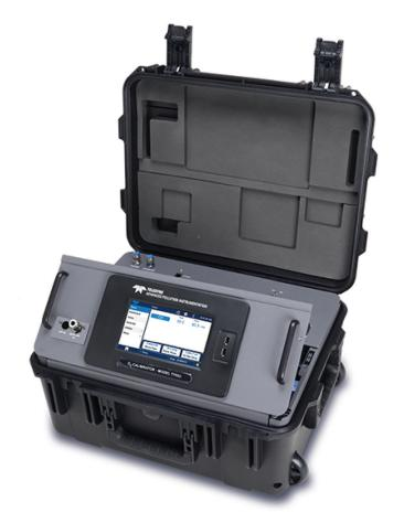
The Model T753U portable photometric O3 calibrator is designed to meet the requirements for low level ozone calibrations and audits, which requires stable, repeatable ozone generation at levels far below the capability of standard ozone calibrators. The Model T753U provides a proven minimum ozone concentration of 2 ppb with exceptional accuracy and stability.
