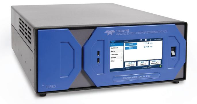
The Model T102 TRS analyzer uses the proven UV fluorescence principle to measure Total Reduced Sulfur at levels commonly required for ambient air monitoring.
