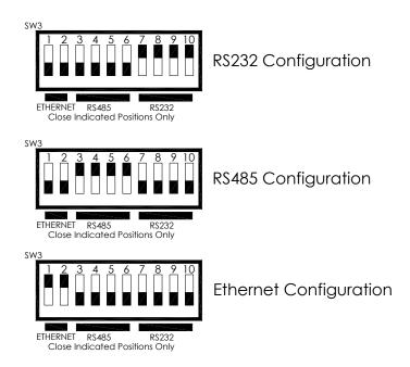
Figure 8-1: COM Configuration Jumper Settings (SW3)
