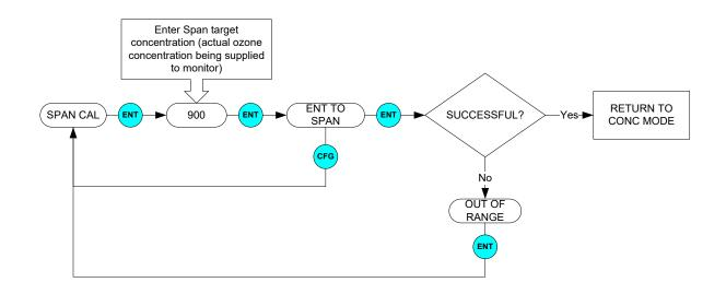
Figure 7-4: Span Cal Menu
