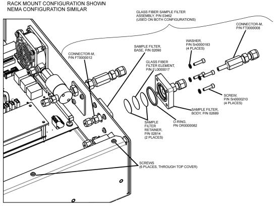
Figure 9-3: Internal Particulate Filter Replacement
