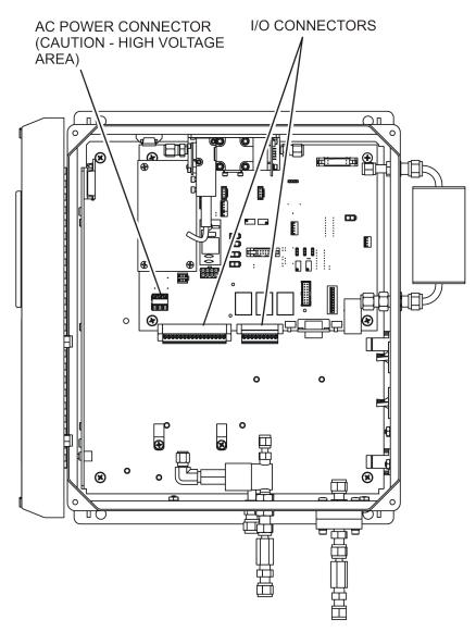
Figure 4-6: NEMA Electrical I/O Connections
