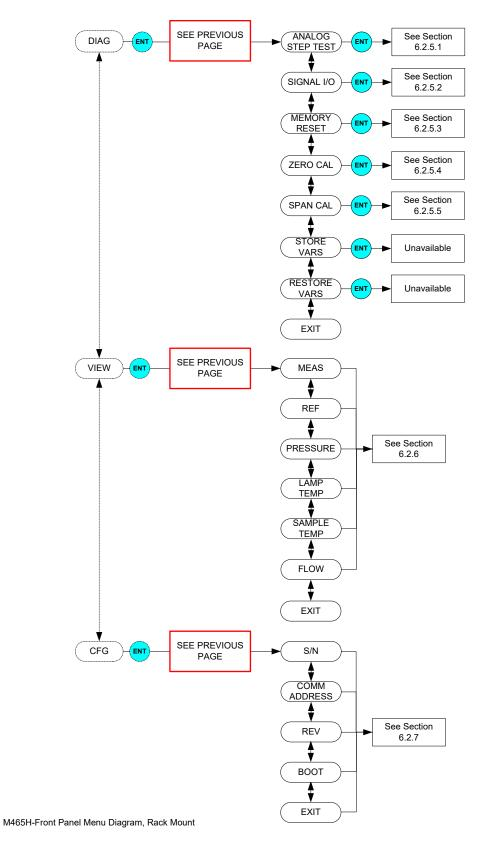
Figure 7-3: Front Panel Menu Diagram
