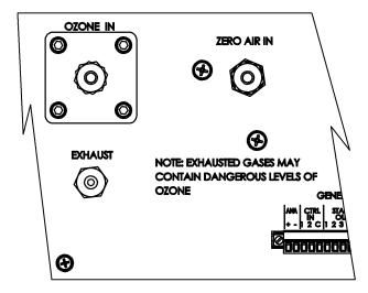
Figure 4-3: Pneumatic Connections, Rack Mount Configuration
