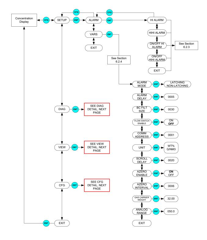
M465H-Front Panel Menu Diagram, Rack Mount
