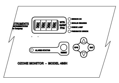
Figure 7-1: Front Panel Display
