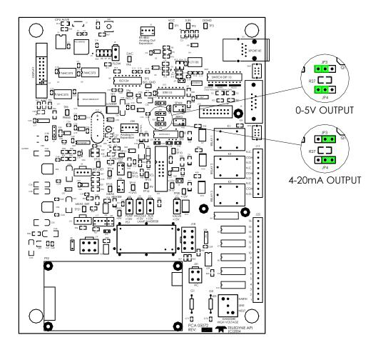
Figure 9-4: Mainboard – Analog Output Configuration
