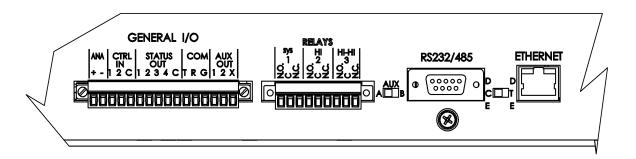
Figure 4-5: Rear Panel Electrical I/O Connections
