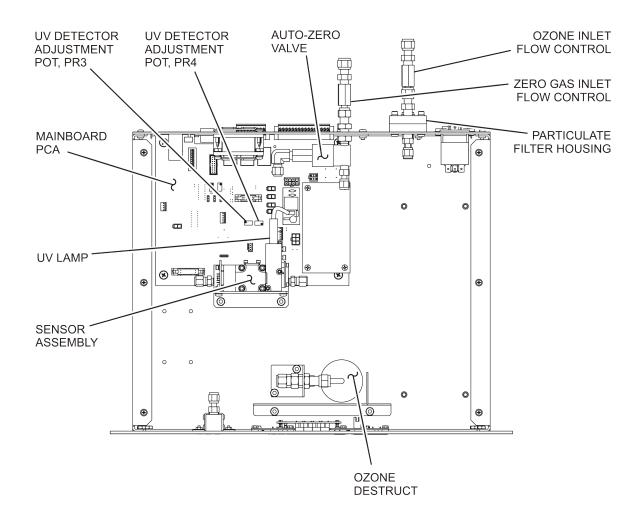
Figure 9-1: Instrument Layout, Rack Mount Configuration
