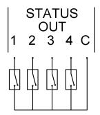
Figure 4-8: Status Output Schematic
