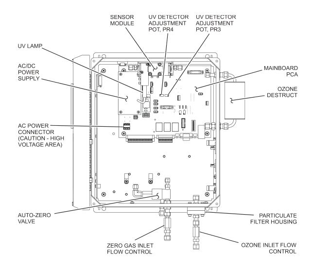
Figure 9-2: Instrument Layout, NEMA Configuration
