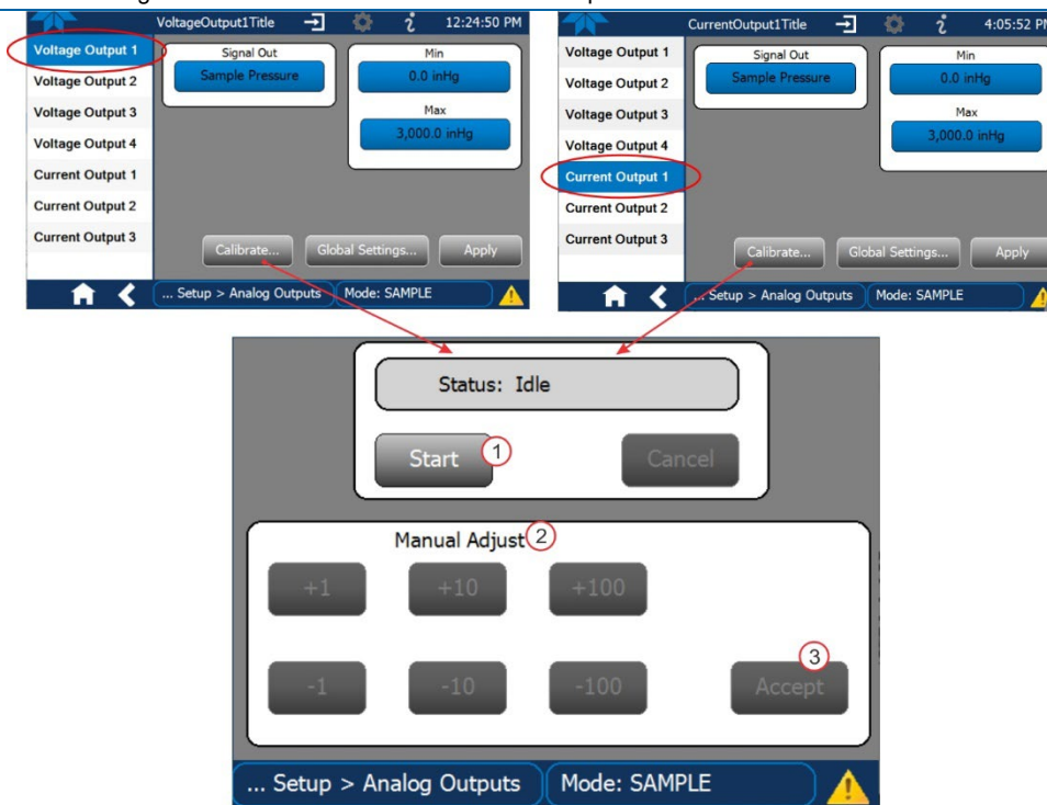
Figure 2-35. Analog Output Calibration, Voltage or Current
