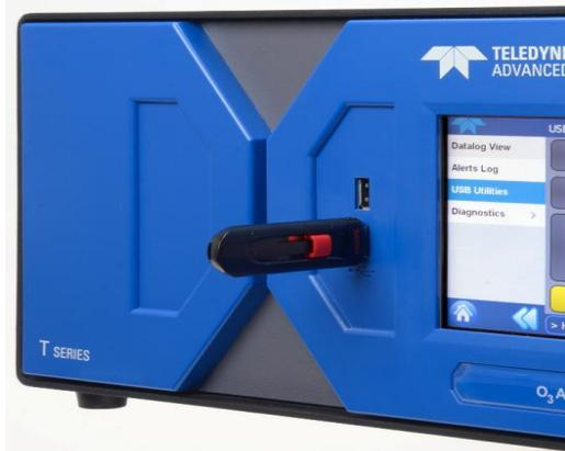
Figure 2: T Series front panel USB Port
