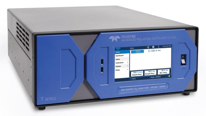
Using a gas filter correlation wheel, the Model T360M Mid-Range  $CO_2$  Analyzer measures carbon dioxide by comparing infrared energy absorbed by a sample to that absorbed by a reference gas according to the Beer-Lambert law. This design produces excellent zero and span stability and high signal to noise ratio, allowing excellent performance over a wide concentration range, making this instrument an ideal choice for  $CO_2$  reporting requirements associated with dilution CEMS.
