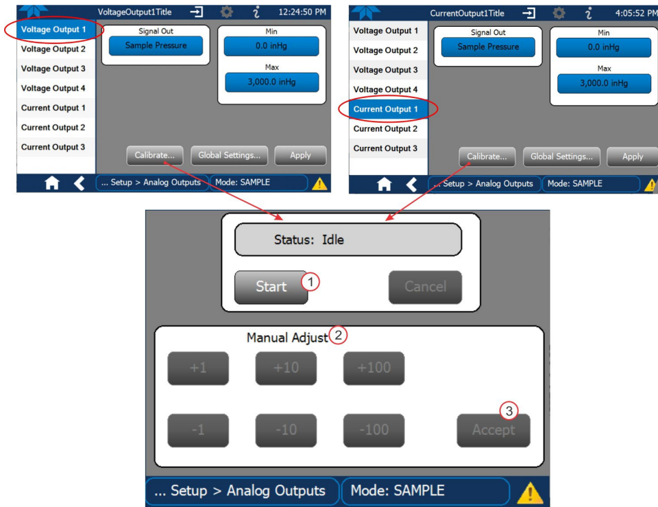
Figure 2-43. Analog Output Calibration, Voltage or Current
