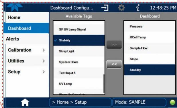
**Figure 2-43. Dashboard Display and Configuration**
