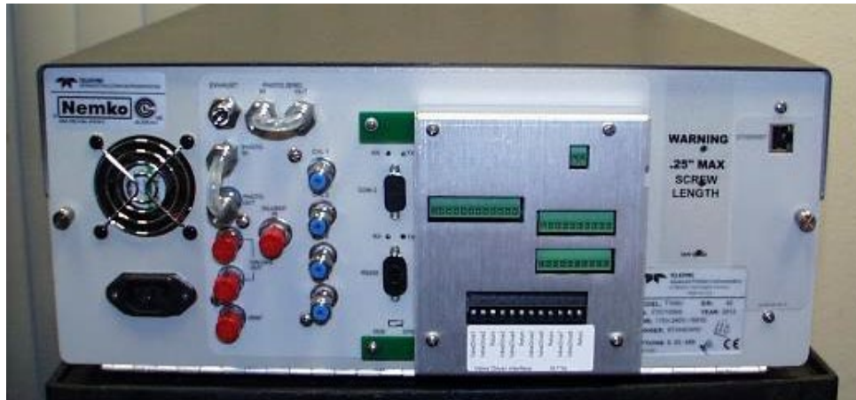
Figure 2-10. Calibrator Rear Panel Valve Driver Installed (without PSM)
