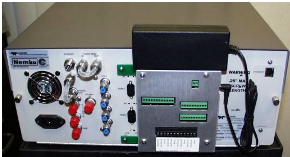
Figure 2-9. Calibrator Rear Panel Valve Driver Installed (with PSM connected to JP1)
