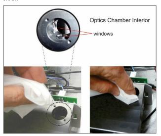
Figure 5-6. Maintenance: Optics Chamber Windows
