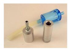
Figure 4-1. Leak-Check/Flow-Audit Adaptor Kit
