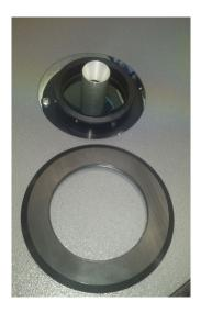
Figure 2-9. Collar for Lower Flange
