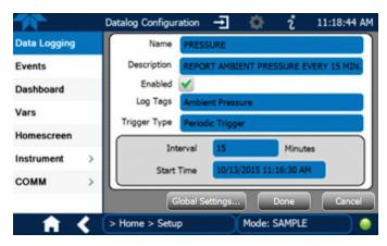
Figure 3-11. Datalog Configuration, Existing Log
