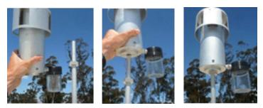
Figure 2-18. T640 Inlet and Sample Line Assembly
