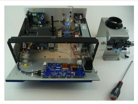
3. Locate the optical cell nozzle, the cup at bottom of optics chamber and its tubing, and the Relative Humidity and Temperature (RH/T) sensor.
