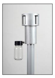
Figure 5-1. T640 Inlet (standard)
