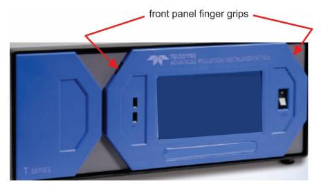
Figure 5-3. Opening the Front Panel
