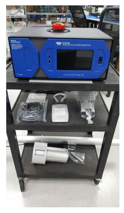
Figure 2-1. T640 Typical Set of Included Hardware
