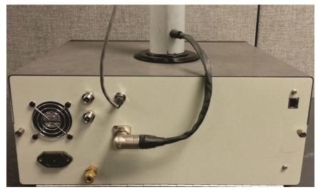
Figure 2-12. Ambient Temperature Probe and ASC Connections (T640 with 640X Option shown)
