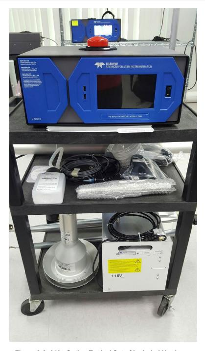
Figure 2-2. 640x Option Typical Set of Included Hardware
