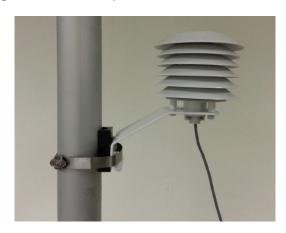
Figure 2-15. Ambient Temperature Sensor Probe Installed into Radiation Shield
